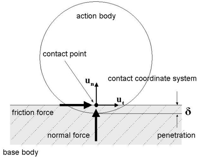
Figure 3 Contact forces between a contact pair
