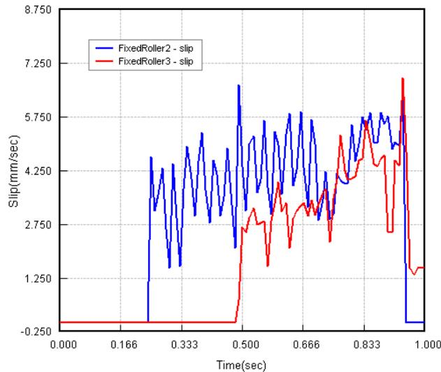
Figure 11 Slip between rollers and sheet
