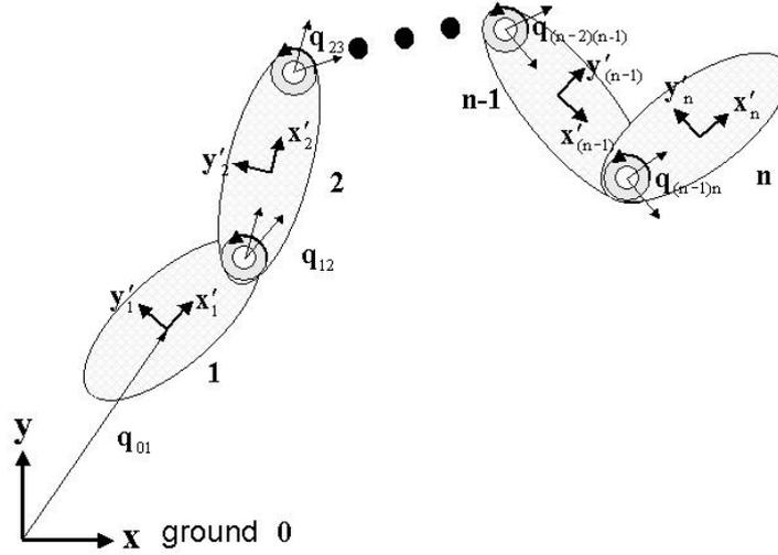
Figure 9 Kinematic relationships between rigid bars of the sheet
