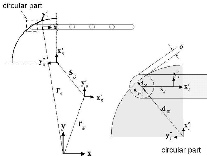
Figure 7 Sheet and arc guide interactions
