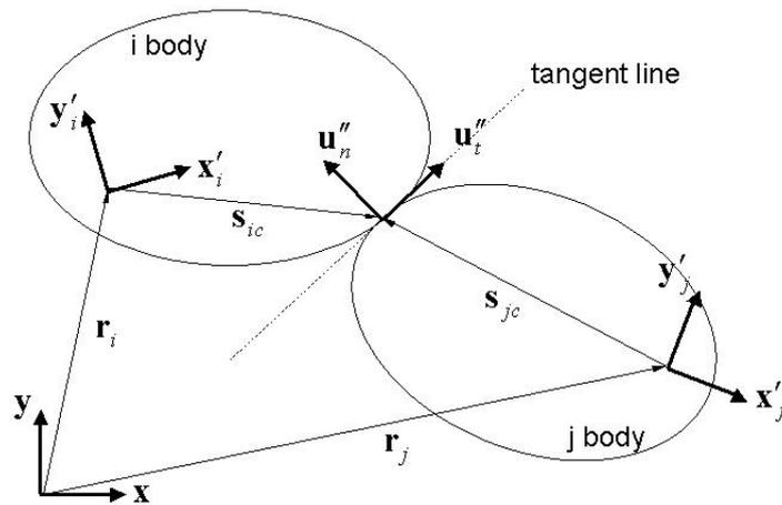
Figure 4 Kinematic notations of a contact pair
