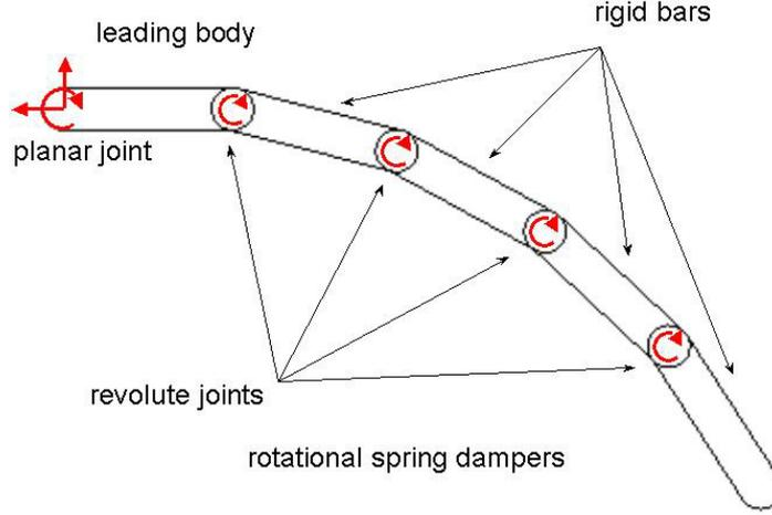
Figure 1 Modeling definition of a two dimensional flexible sheet
