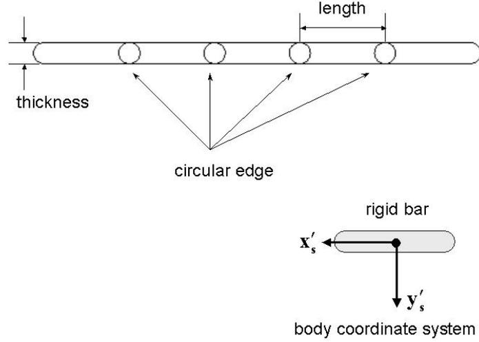
Figure 2 Contact geometry of two dimensional sheet
