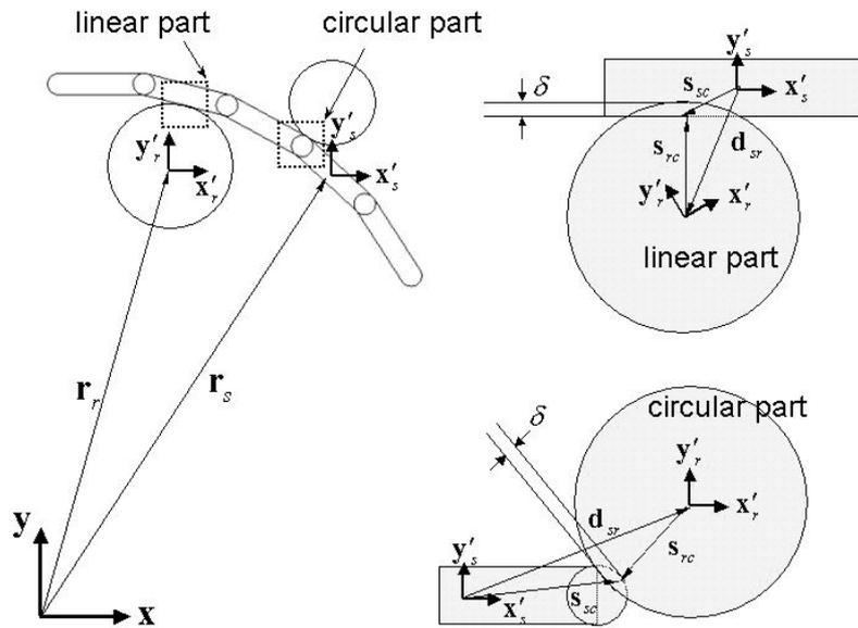
Figure 6 Sheet and roller interaction
